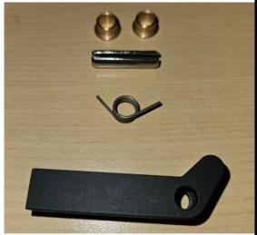
fix my problem. After some time, I figured out a much simpler way to remove the latching arms. At disassembly, I found plastic bushings and a pivot pin that were worn beyond use. After trying to find the bushings, with no luck, I decided the only solution was to make custom bushings. This was the beginning of a repair kit for Retro Thunderbirds that Ford does not supply. I currently can supply: Bushings, Pivot Pins, Pivot Arms, Springs, and instructions to disassemble and assemble.
